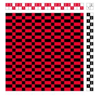
be substituted as in the fabric shown below. The drawdown is simply that of plain weave.
